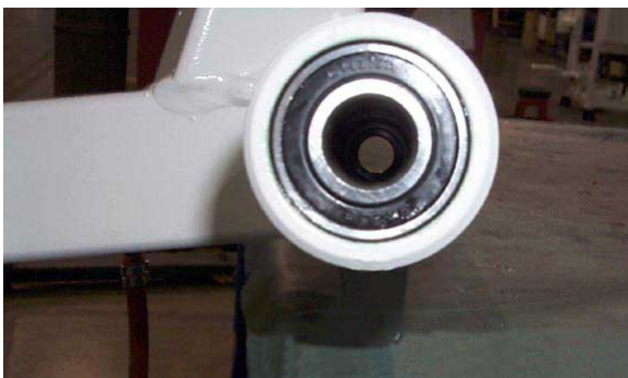
Cybox uses Loctite® RC™ 680 Retaining Compound to fill the gaps between the tubing and the slip fit bearing on pivot arms of their line of VR-2 variable resistance strength-training equipment.
